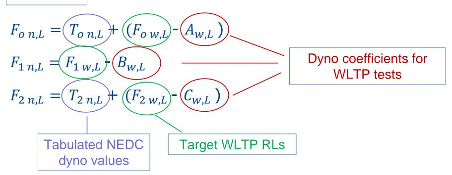
When for WLTP RLs are used default values (or RLMF) the following procedure for NEDC shall apply.
